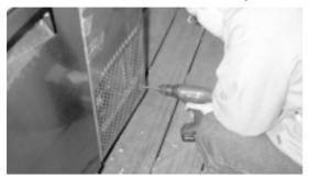
B. Lift up the front grille panel and pull it out. Cut the silicon off around the cabinet front cover using a knife and pull it out.
