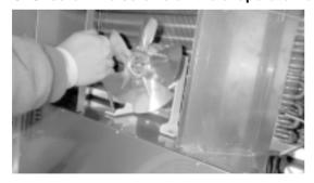
D. Disconnect the evaporator fan motor from the main harness. Replace the old one with new.
