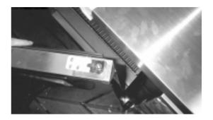
B. Lift the door. Replace the old one with new. Insert the door hinge top into the door bush. Angle between the door line and the hinge bracket line is 90° as pictures below.
