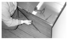
C. Disconnect the cabinet frame heater from the main harness. Relpace the old one with new.
