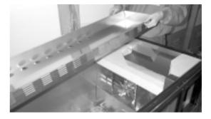
E. There is a insulator that guides cold air flow into the air duct panel. Pull it out. You can see the duct panel which shape is '\(^{\strue{\sigma}}\)'.
