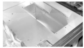
F. Unscrew the screws on the air guide panel (B) and (C).
