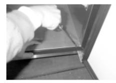
B. Separate the end of the cabinet frame cover and pull it out continuously to the end of the other side.
